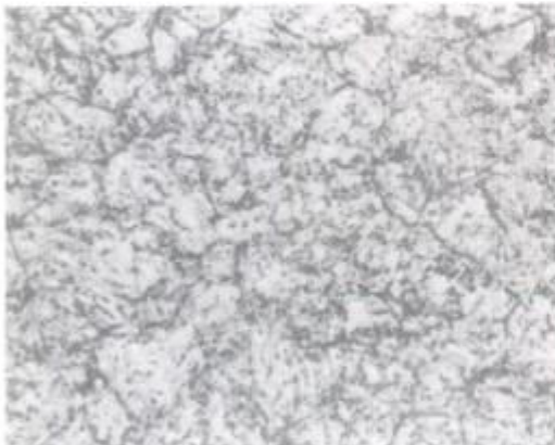
Quenched and tempered structure of H 13 showing finely dispersed spheroidal carbides in ferrite matrix (Magn 1000x)
